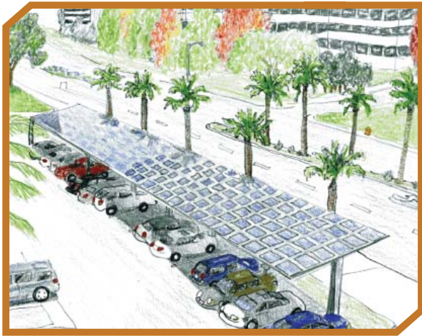
PV on covered parking structure.
